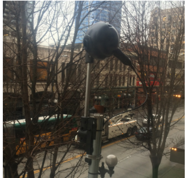
Passive Infrared Pedestrian Detector
