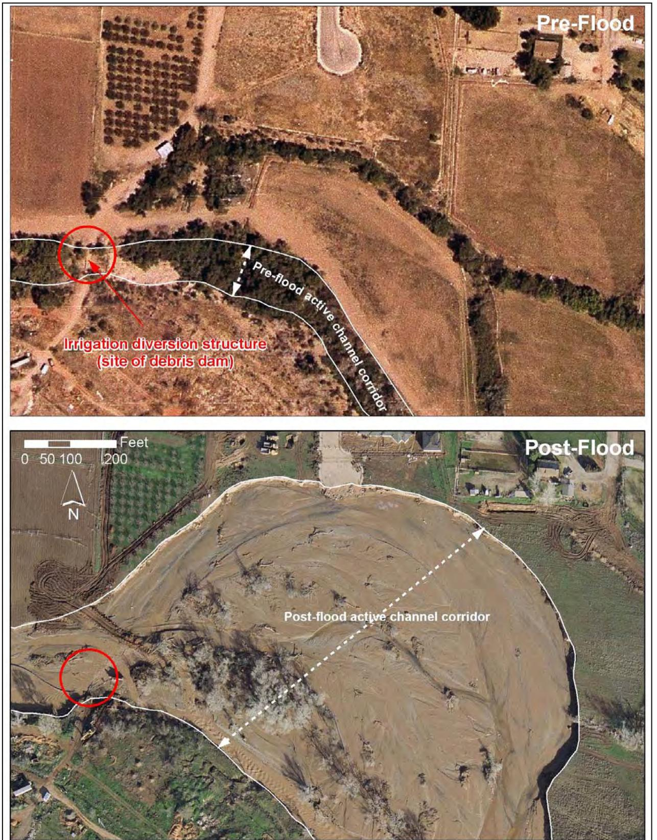
Figure 10. Debris dam at irrigation diversion structure
