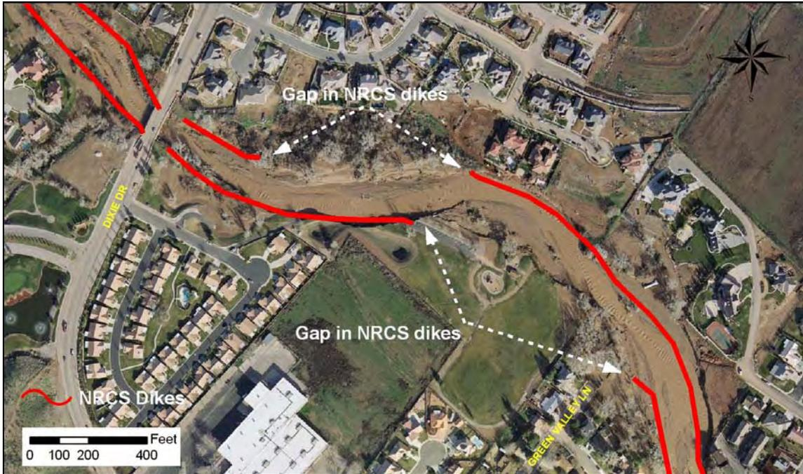
**Figure 27. Examples of gaps in NRCS dikes**
