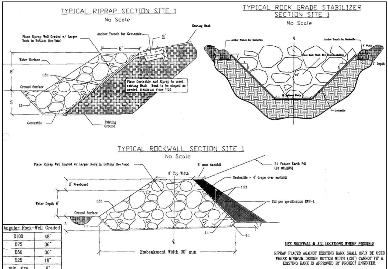
Figure 22. NRCS structures typical designs
